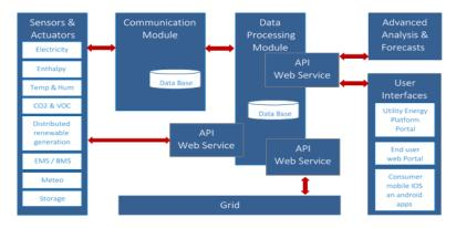
Fig. 1: System architecture.
