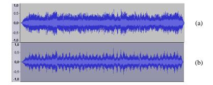
Fig. 6: a) Original sound; b) sound after tremolo filter.
